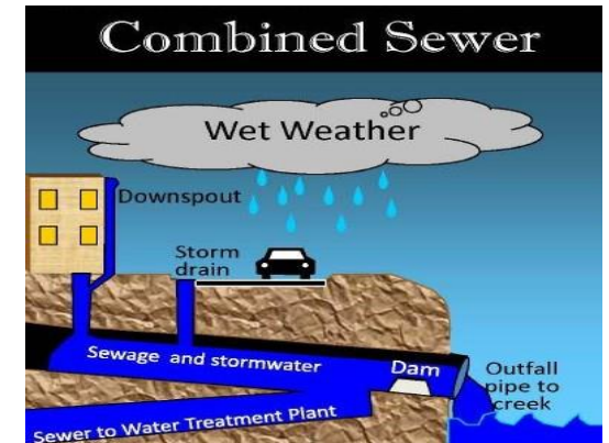
Pictured is a wet weather visual of a combined sewer overflow system.
